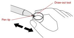
Figure 4-5 Replacing the pen tip
